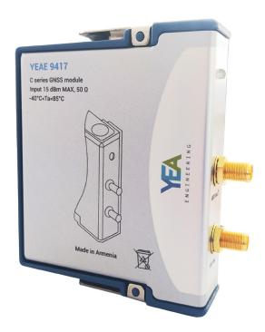
The YEA 9417 is a concurrent GNSS receiver module for NI C series platforms. It can receive multiple GNSS systems signal (e.g GPS/QZSS, GLONASS, BeiDou). Due to dual-frequency RF front-end architecture, two of the three signals (GPS L1C/A, GLONASS L1OF, and BeiDou B1) can be received and processed simultaneously.
